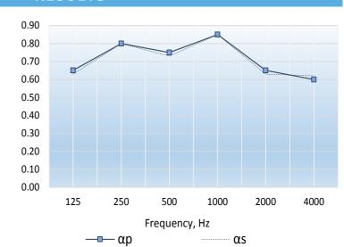
Single figure rating :  $\Omega\omega$  0.70(L) In accordance with BS EN ISO 11654: 1997
