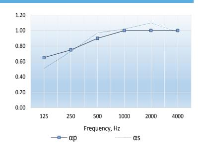
Single figure rating :  $\Omega\omega$  0.95 In accordance with BS EN ISO 11654: 1997
