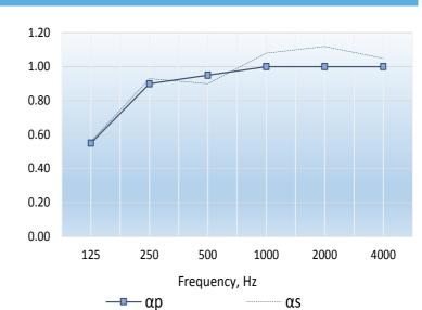
Single figure rating :  $\Omega_{\omega}$  In accordance with BS EN ISO 11654: 1997
