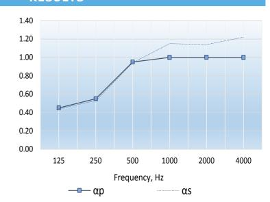
Single figure rating :  $\Omega\omega$  0.85(H) In accordance with BS EN ISO 11654: 1997
