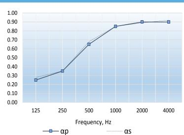
Single figure rating :  $\Omega_{\omega}$  0.65(H) In accordance with BS EN ISO 11654: 1997
