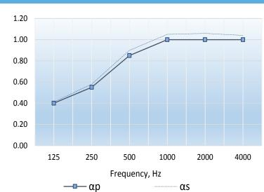
Single figure rating :  $\Omega_{\odot}$  0.85(H) In accordance with BS EN ISO 11654: 1997
