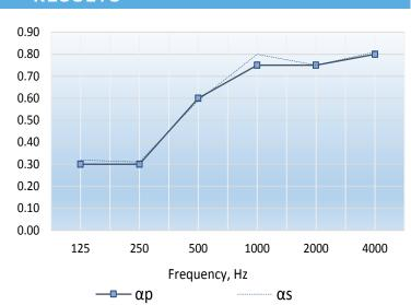
Single figure rating :  $\Omega_{\odot}$  0.60(H) In accordance with BS EN ISO 11654: 1997
