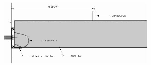
The Nexus profile can be used with support connections when installing a floating perimeter and is easily cut on site to suit conditions.
