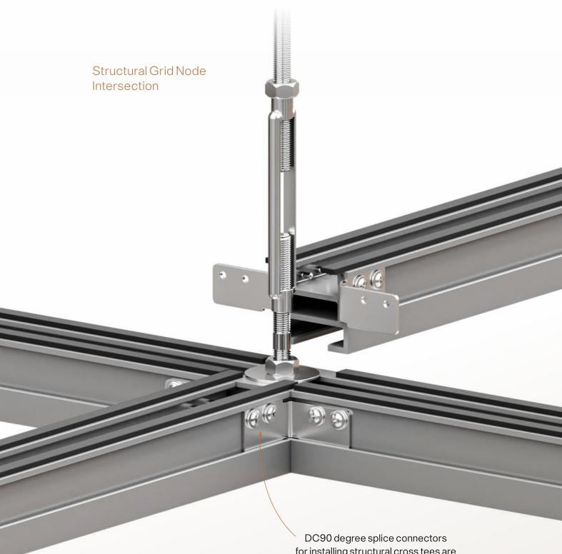
DC90 degree splice connectors for installing structural cross tees are removeable allowing easy positioning and in-situ adjustment.
